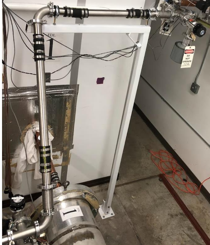
Figure 36: End Support of Manifold to Vacuum Pump
